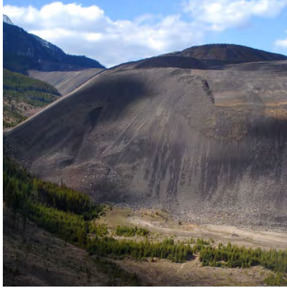
A Conventional Waste Rock Dump
